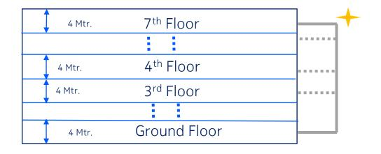
12F (Vertical Riser Cable runs from Ground Floor connecting till 7th Floor Access Switch and other VR cable for redundancy
