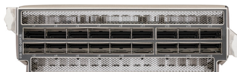
18-connector 100G QSFP28 MDA-s
